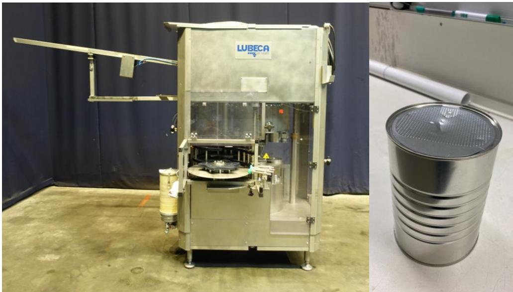
Can closing machine. Stand-alone and fully automatic. The Lubeca is suitable for seaming lids onto cans, equipped with 4 seaming stations. Working principle: The incoming cans are synchronized to the machine by a specially constructed infeed gear-wheel. An electro-pneumatic system manages the required feed of lids as required ("no can –no lid").
